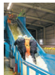
実物大階段模型(流水階段) Scale model of a staircase (Water flowing staircase)
