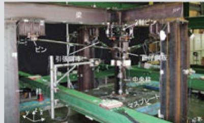
当分野で開発した低負荷耐震補強機構の動的2軸載荷実験 Dynamic bidirectional loading test of Minimal-Disturbance Arm Damper developed by our group
