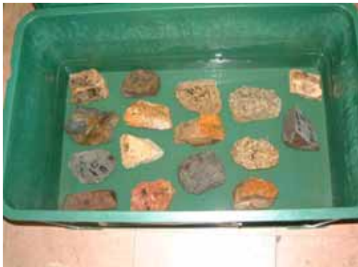
Photo 2 Example of stones in water in order to be saturated. This condition was kept for at least 1 week through some months.
