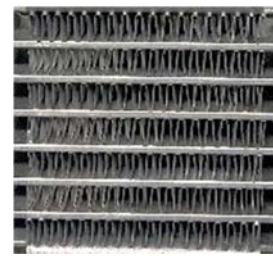
Fig.2 Front view of the corrugated fin heat exchanger
