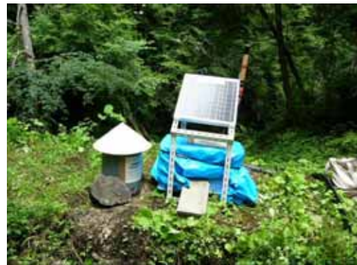
Photo.3 A total set of our seismic observation system
