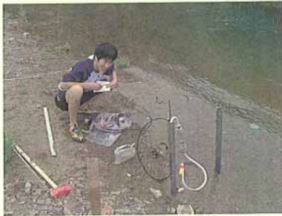
Photo 3 Permeability test in the field.
