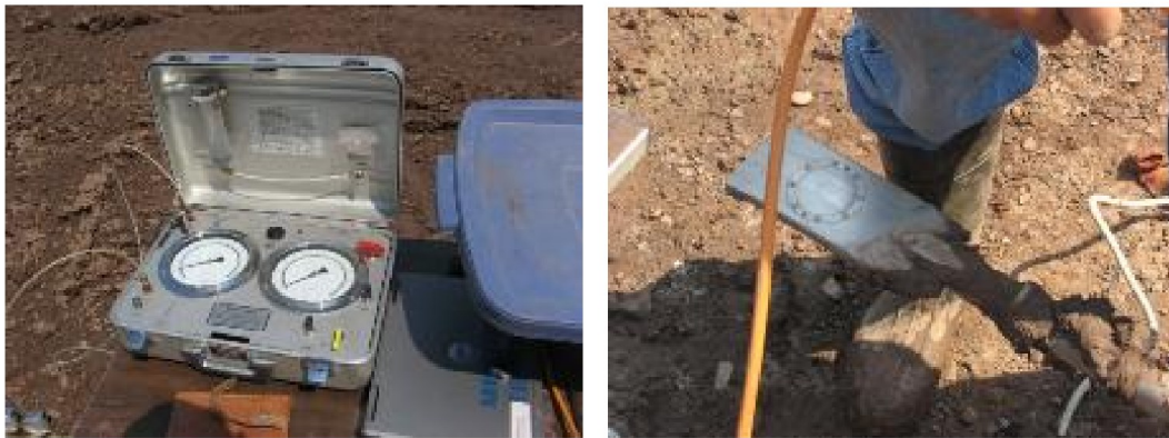
Figure 2.6. Dilatometer control panel and blade in DMT test (Ruffing et al., 2015).
