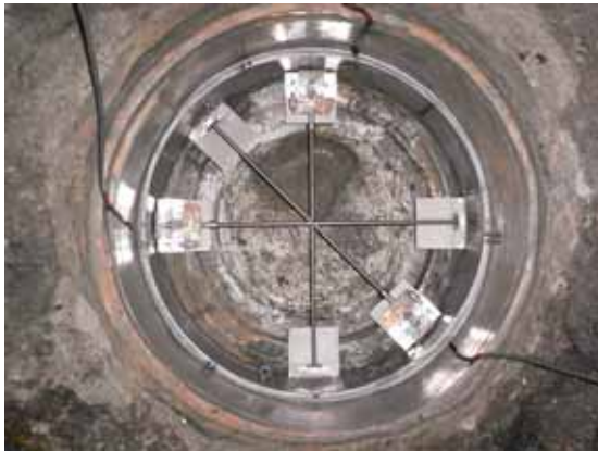
Photo 3 The short span strainmeter set into the hole
