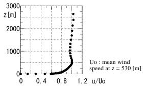
Fig. 10 Mean wind speed profile at the inlet boundary for LES
