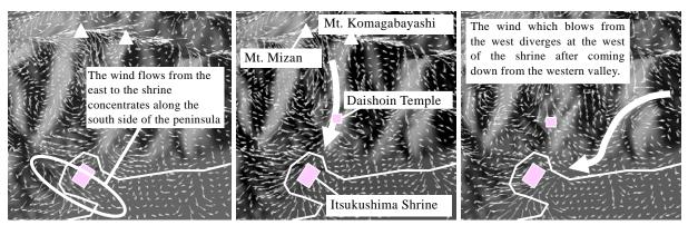
a. East wind at the shrine b. South wind at the shrine c. West wind at the shrine Fig. 14 Instantaneous wind velocity vector fields around Itsukushima Shrine at 10m
