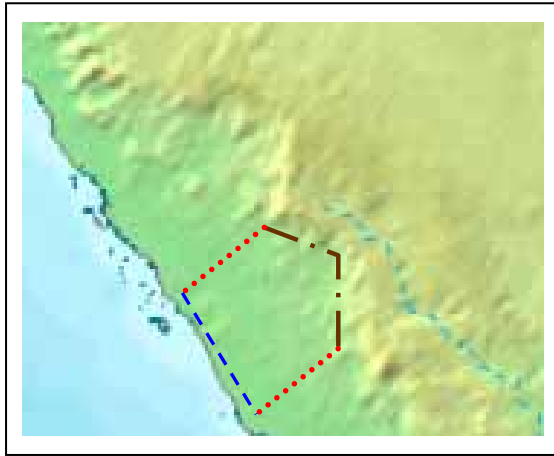
Fig. 13 Typical boundary conditions at the western coast of Saudi Arabia: (no-flow boundaries are dotted)
