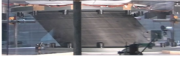
Figure 1. Laminated high damping rubber bearing (HDRB) undergoing lateral loading in the test facility.
