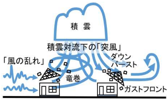
Fig. 1 Origin of strong wind which causes damage on houses and buildings
