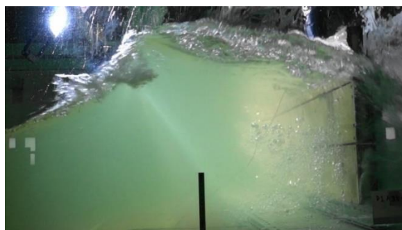
(3) The wave is reflected by the Door (0.9s after)
