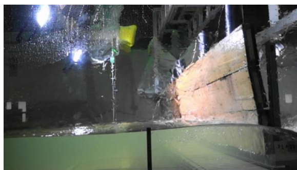
(4) The wave has gone and the door starts to fall down (2.1s after)
