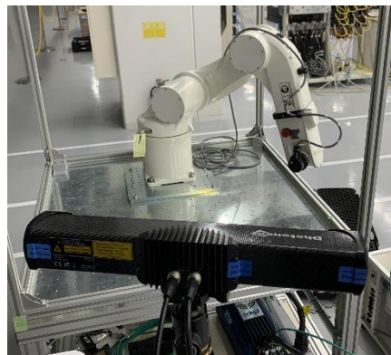
Fig. 9. Measurement of point cloud data with a 3D scanner.
