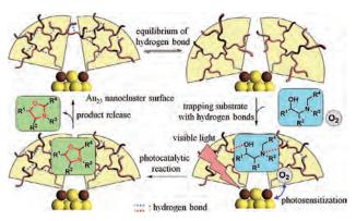
Figure 2. Schematic illustration of photocatalytic oxidation of amino alcohol accelerated by supramolecular reaction field constructed of peptide dendron thiolates on  $Au_{25}$  nanocluster.
