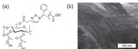
Figure 1. (a) Chemical structure of cellulosic BB and (b) TEM image of its annealed bulk film (PCL: DS = 1.5, DP = 100; PS: DS = 0.75, DP = 90).
