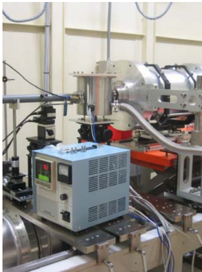
Figure 1. Experimental set-up of the present in-situ measurements. The sample chamber, center, was evacuated by a turbo molecular pump during in-situ measurements. The upstream and downstream pipes with lower vacuum were separated from the sample chamber.
