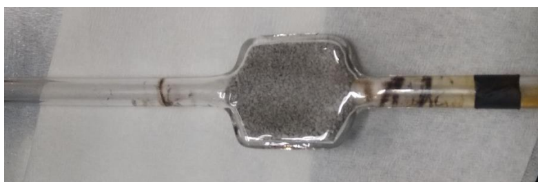
Figure 7 Photograph of the sample cell after the reaction at 623 K with the Pd(0.5)/Ga 2 O 3 sample
