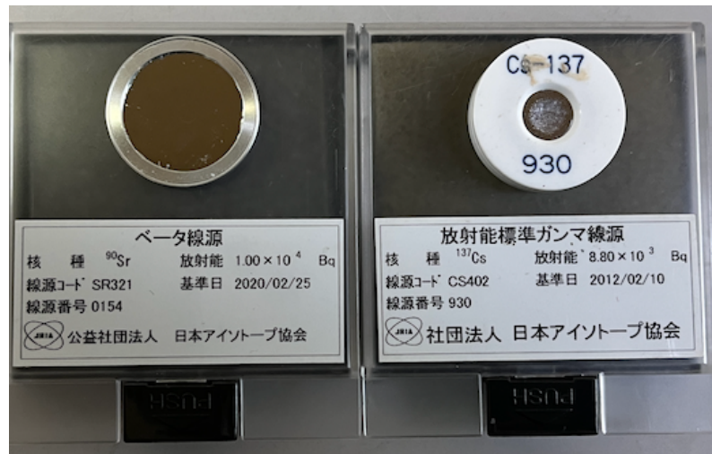
Fig. 3-4 Standardised \beta - and \gamma -ray radiation sources with radionuclides of ^{90}\text{Sr} and ^{137}\text{Cs}
