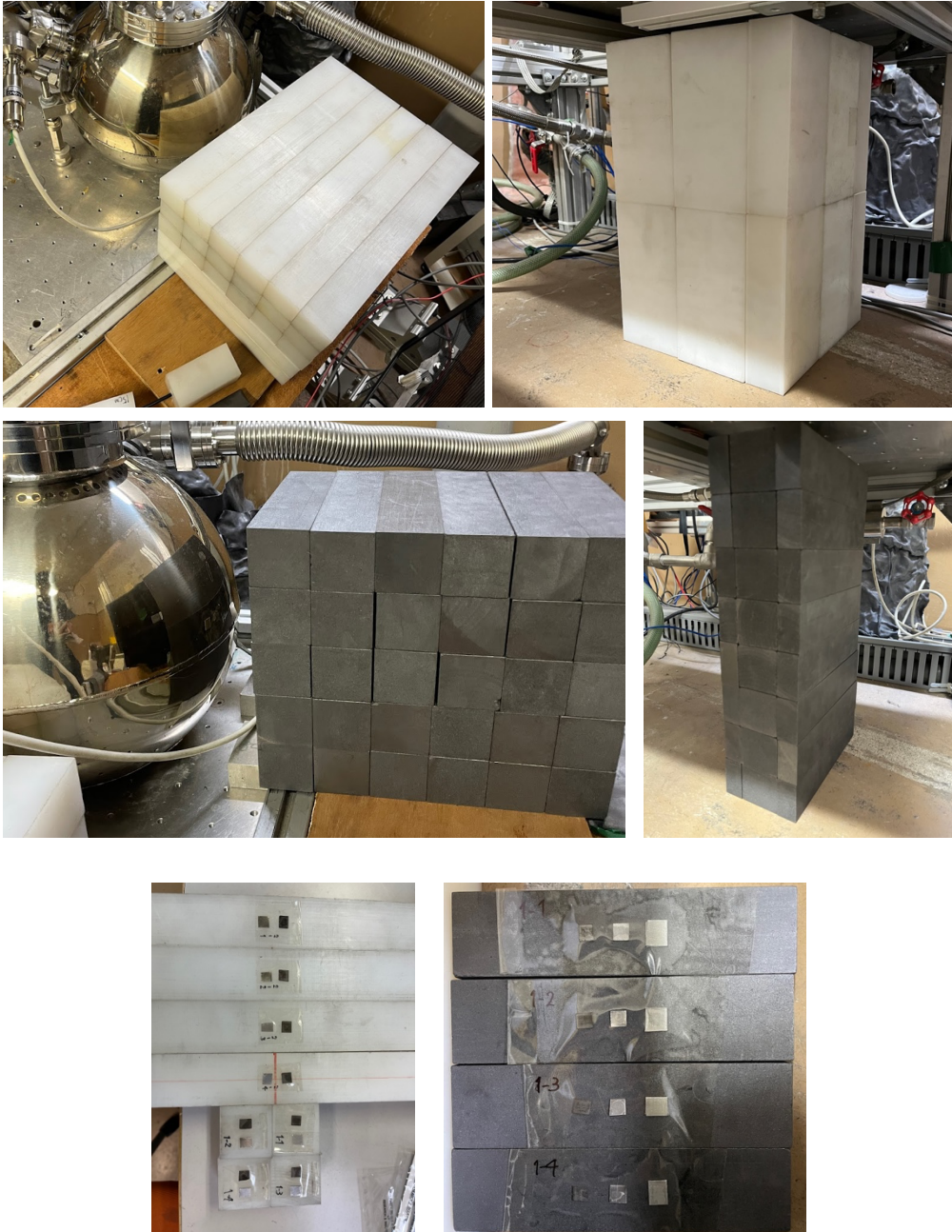
Fig. 3–2 Configuration of mock-up experiments: mock-ups composed of polyethylene blocks (upper) and graphite blocks (middle), and material foils attached to each mock-up block (lower)
