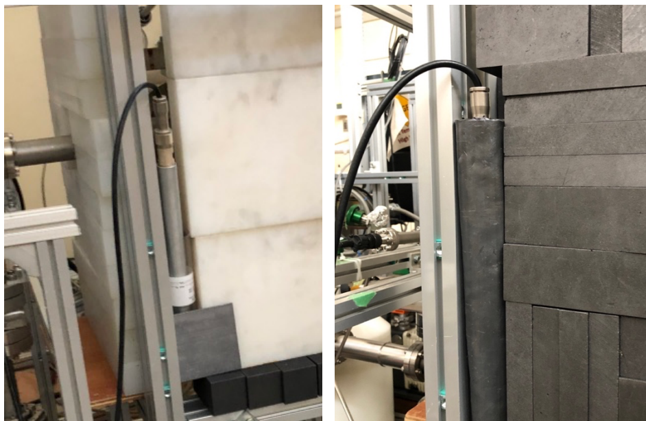
Fig. 2–9 Installed position of the ^3\text{He} neutron counter without lead sheet (left) and with lead sheet of 2 mm thickness rolled twice (right)
