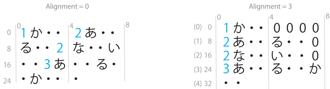
Figure 2.3: String storage alignment example. Dots are additional bytes used by UTF-8 encoding for the respective symbols. Storage with alignment=3 can be indexed using the numbers in brackets.
