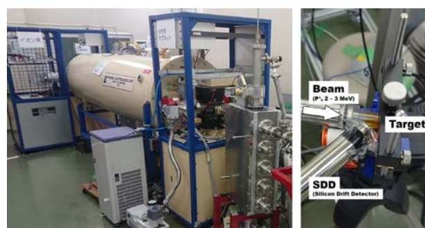
Fig. 2. In-air PIXE analysis system at TCU-Tandem.
