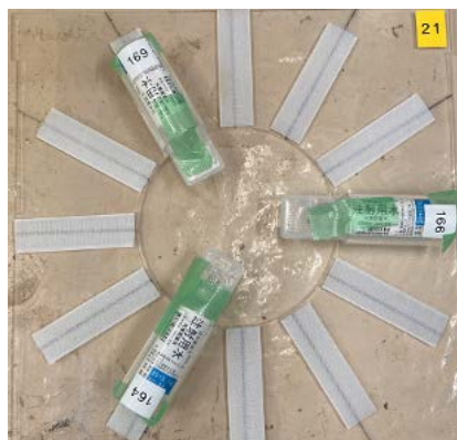
Figure2: The mouse is placed in the irradiation hole in the form of a radial projectile.
