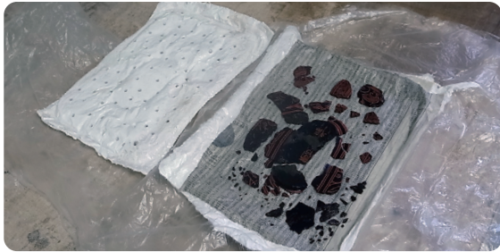
3. The lacquer fragment was soaked in water. In water, the lacquer fragment was free, the warp was removed off it. Furthermore, the dirt (mud) was removed by ultrasonic cleaning.
