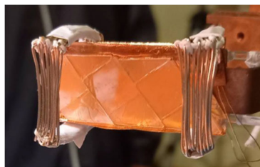
Fig.3 The picture of YSZ and coil used in HIMAC.
