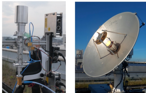
16 - 64 GHz wideband feed under developing for the radiometer(left), and 2.4 m antenna(Right) of NICT with 3.2 - 16 GHz weideband feed for VLBI, which will be used for the radiometer with new feed.
