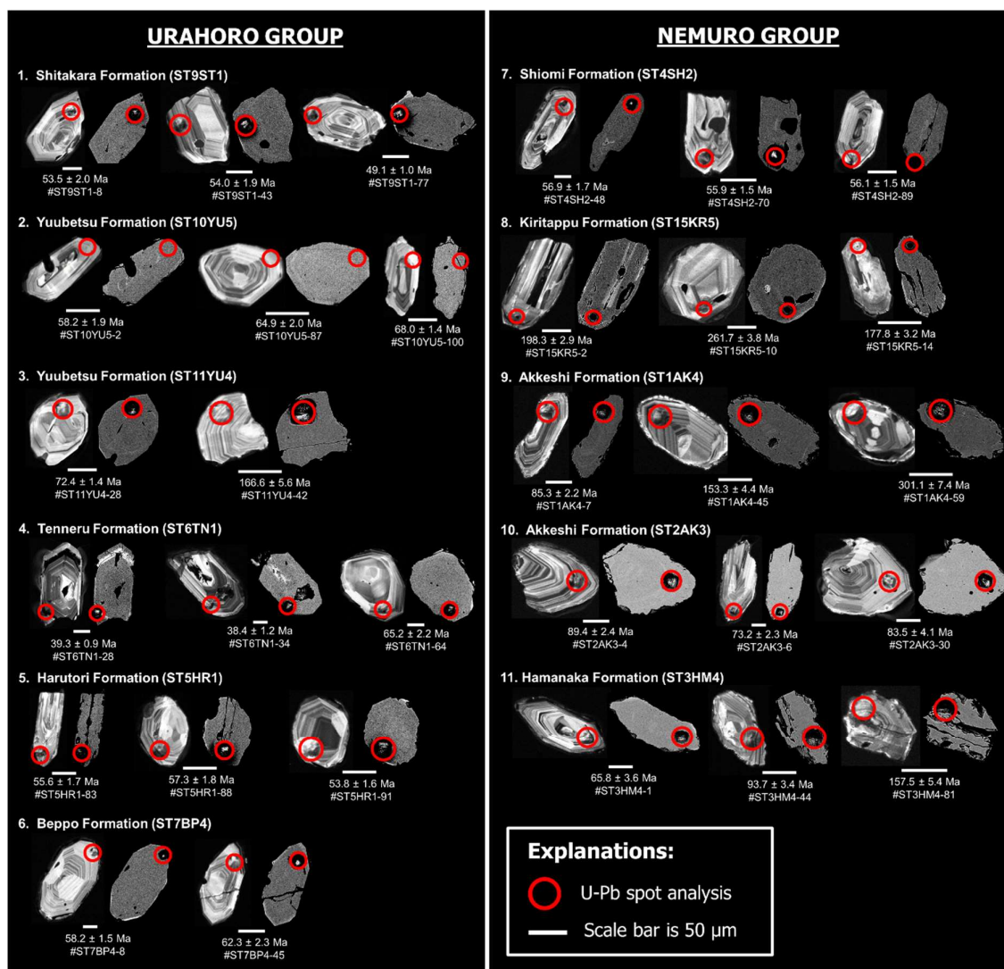
Figure 8. Cathodoluminescence (CL) and backscattered electron (BSE) images of selected detrital zircon for the Urahoro Group (left) and Nemuro Group (right). Red circles indicate the locations of the U-Pb spots. White scale bars are 50 \mu m long.
