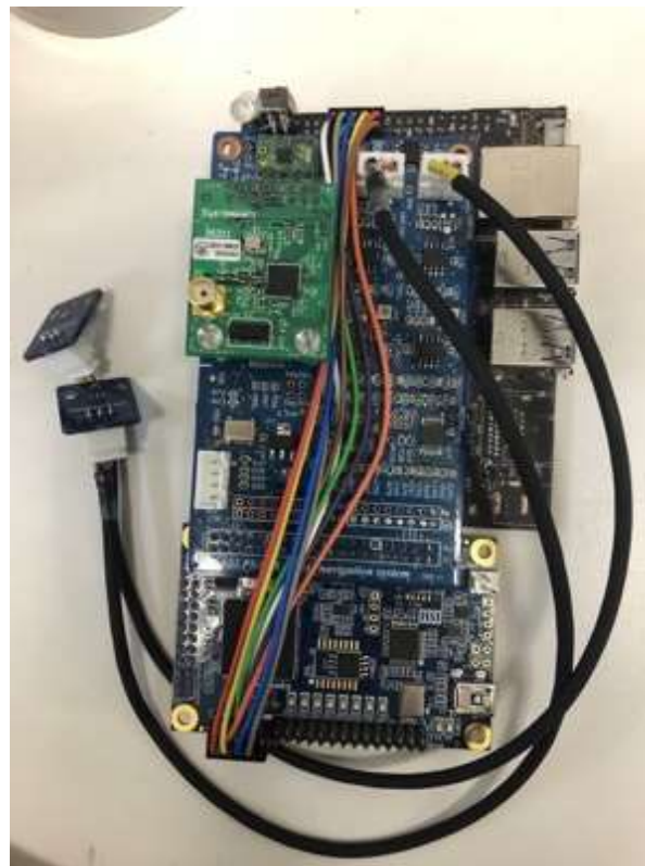
Fig.2.8 Wireless receiving unit
