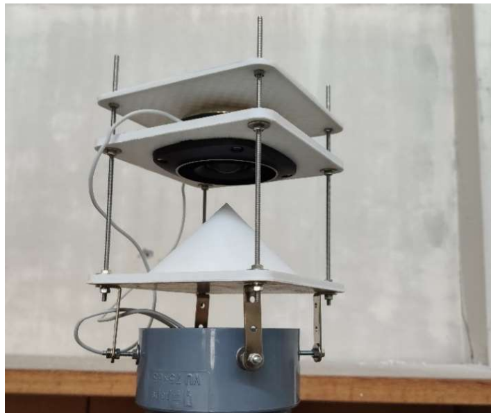
Fig.2.5 Speaker with 3D printed cone
