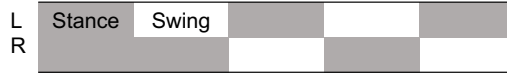
Figure A.2: The contact pattern of the iCub walking. L denotes the left foot in contact and R does the right foot in contact.
