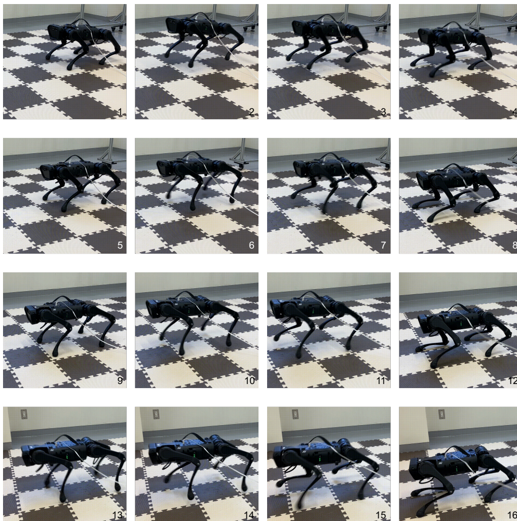
Figure 7.9: Snapshots of successive four-times dynamic jumping of quadruped robot Unitree A1 by the proposed whole-body MPC-STO. A supplemental video is found at https://youtu.be/SureDVDFbfM .
