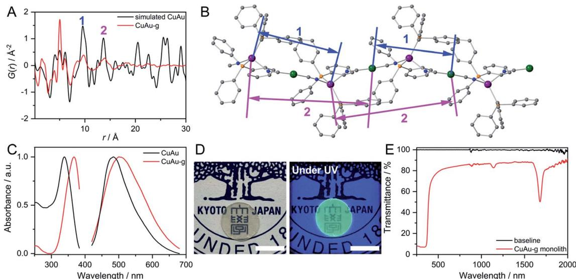
Fig. 2 (A) PDF profiles of simulated **CuAu** and **CuAu-g** at 25 °C. (B) Atomic pairs corresponding to peak 1 and 2 in the PDF profile of **CuAu**. Grey, blue, orange, violet, and green are C, N, P, Cu, and Au, respectively. (C) Excitation and emission spectra of **CuAu** and **CuAu-g** at 25 °C. (D) Transparent monolith of **CuAu-g** made by hot-pressing with/without UV light. Scale bar is 1 cm. (E) Transmittance of the **CuAu-g** monolith from 250 nm to 2000 nm.
