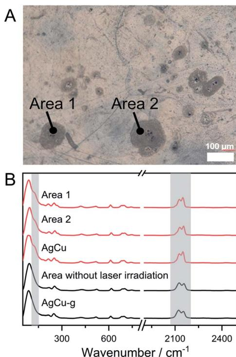
Fig. 3 (A) Surface of the **AgCu-g-CuSO<sub>4</sub>** monolith under the microscope. Areas 1 and 2 are irradiated using a 47  $\mu\text{m}$  size laser. Other grey spots are also crystallized domains. (B) Confocal Raman spectra at areas 1 and 2, and the area without laser irradiation. Spectra of pure **AgCu** and **AgCu-g** are also shown.
