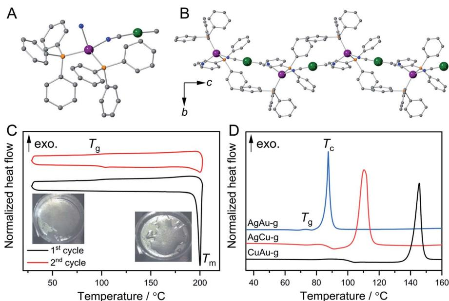
Fig. 1 Crystal structures of **AgAu** (A) in the  $\text{Ag}^+$  coordination sphere and (B) 1D chains along the  $c$ -axis. Grey, blue, orange, violet, and green are C, N, P, Ag, and Au, respectively. (C) First (black) and second (red) DSC upscan/downscan cycles of **CuAu**. Melting temperature  $T_m$  and glass transition temperature  $T_g$  are shown. (D) First DSC upscan of  $\text{M}^{\text{N}}\text{M}^{\text{C}}\text{-g}$  from 35 to 160 °C. The heating rate is 10 °C  $\text{min}^{-1}$ .
