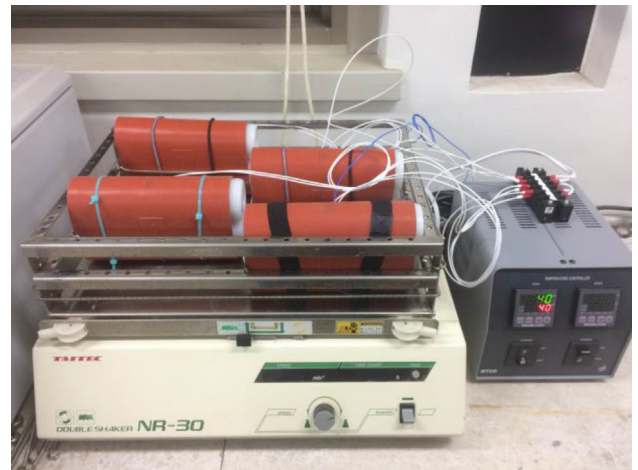
Fig. 4. Batch leaching tests under the shaking conditions using a temperature control system.
