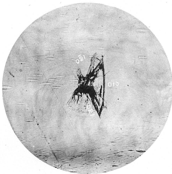
Fig. 1. A triangular tear-figure on (110) of aragonite, the apex opposite (010). The average apical angle is nearly equal to the angle between (021) and (0 \bar{2} 1). Transm. light. Mag. 60 diam.
