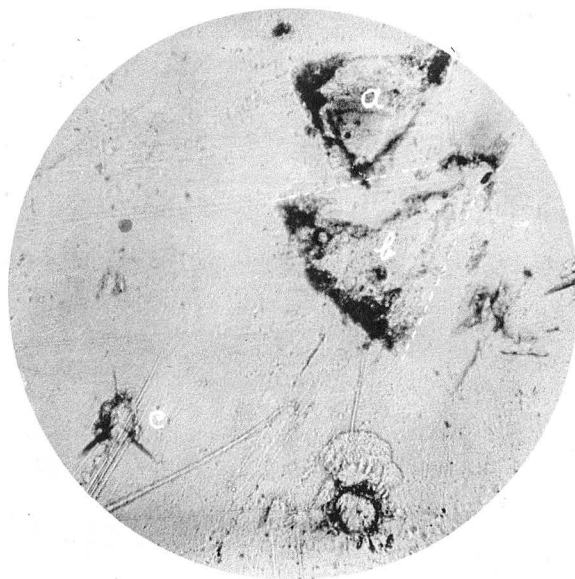
Fig. 1. Triangular (a and b) and three-rayed (c) figures on (III) of alum. Transm. light. Mag. 60 diam.
