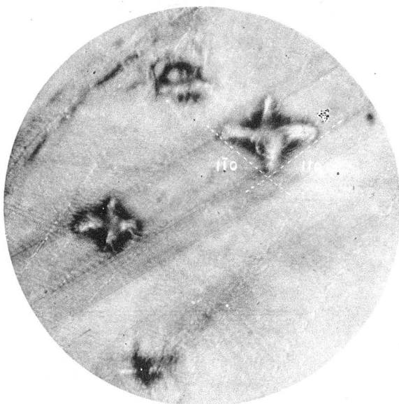
Fig. 2. The same as Fig. 1. The photomicrograph shows an abnormality in the index of refraction, resulted from gliding along the a- and b-axes by the pressure of the needle-point. The picture was taken a little out of focus. Transm. light. Mag. 80 diam.
