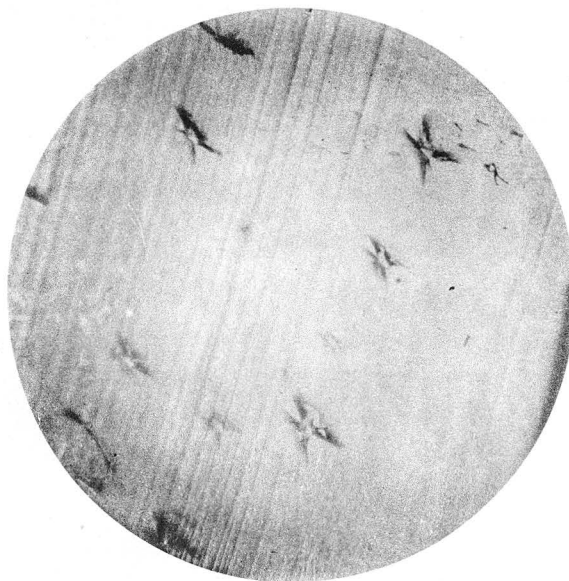
Fig. 2. Tear-figures on the same face as Fig. 1. Various shapes of imperfect figures. The parallel streaks are polishing scratches. Transmitted light. Mag. 60 diam.
