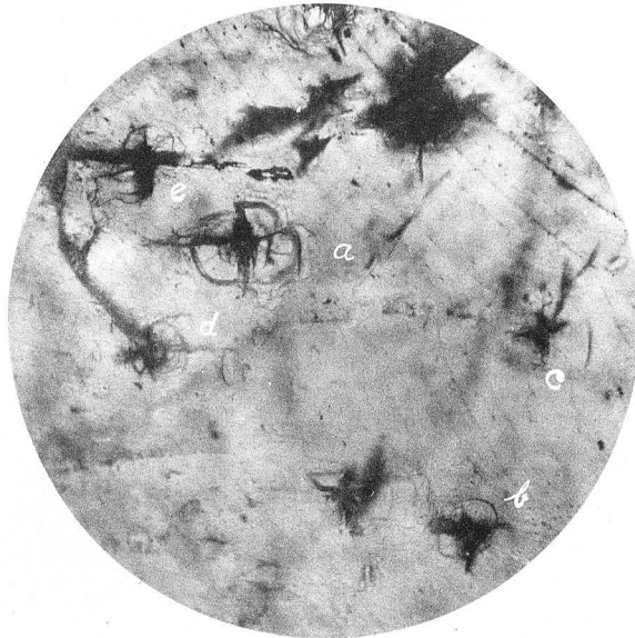
Fig. 1. Tear-figures on \{001\} of wulfenite. a, b and d.....a common type of the figures. The sides are slightly curved giving the figures a rounded appearance. c and e.....a crossed figure, an imperfect one. Transmitted light. Mag. 60 diam.
