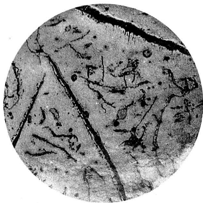
Photogr. No. 60. \times 150 Cast iron furnace cooled.
