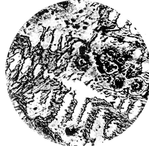
Photogr. No. 6. \times 900 C=3.45%, Si=5.80% Etched with sodium picrate
