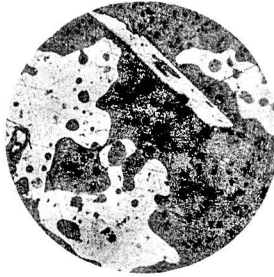
5. CZA 8 (Cu 2.08%, Zn 52.97%) quenched at 350°C. \times 150
