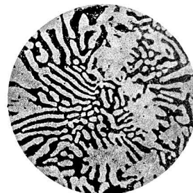
23. CZF 8 (Cu 19.37%, Zn 52.55%) quenched at 350°C. \times 300
