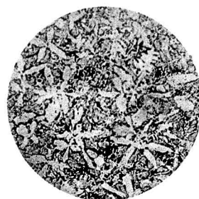
21. CZF 7 (Cu 17.88%, Zn 62.75%) chill cast. \times 250
