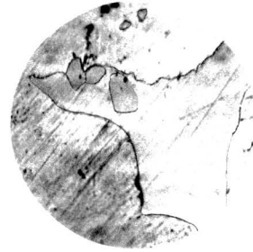
35. ZF 3 (Cu 10.09%, Zn 14.46%) quenched at 350°C. ×750
