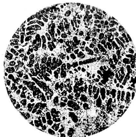
7. CZC 4 (Cu 2.62%, Zn 85.88%) chill cast. \times 170
