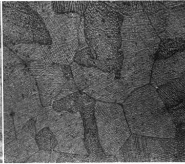
78.8% Copper. Quenched at 500°. Twinned \delta . \times 100 . (Iodine solution)
