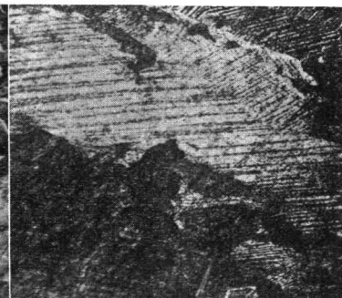
75.0% Copper. Quenched at 500°. \zeta_2 . \times 100 .
