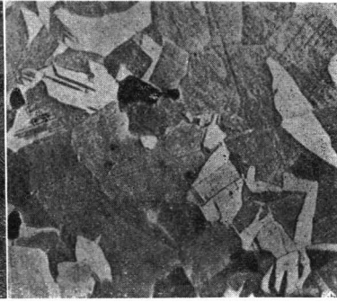
78.0% Copper. Quenched at 610°. \delta . \times 100 . (CuCl 2 solution)
