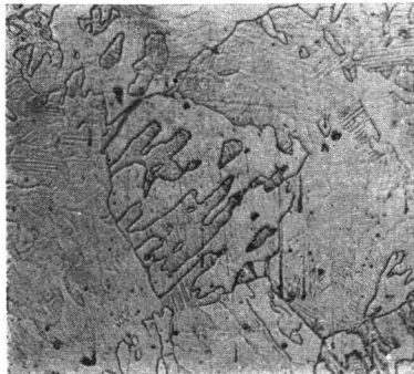
78.0% Copper. Quenched at 500°. Decomposed \delta . \times 100 . (Iodine solution)
