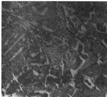
(37) TSA 1220 (68% Cu, 12% Si) Furnace cooled. ζ + ε + Si. × 00.
