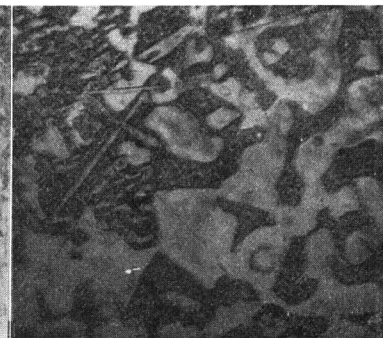
(35) TSA 1005 (85.0% Cu, 10.11% Si) Furnace cooled. \gamma_L + \epsilon_S'' + Si . \times 100 .
