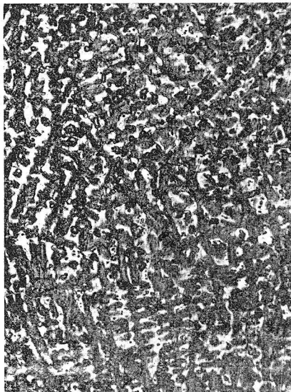
(19) 20% Al, 30% Fe, 50% Cu. \times 150 Furnace cooled.
