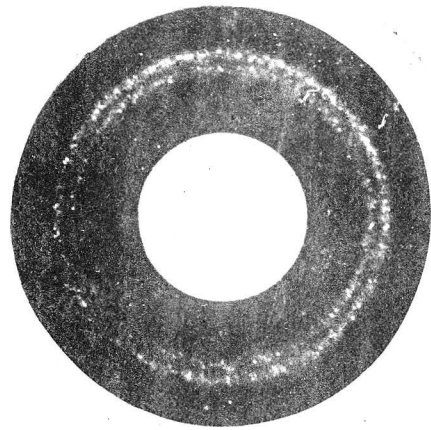
Photo. 16. Specimen H3, \sigma_a = \pm 10 , \sigma_m = -10 , N = 9.02 .
