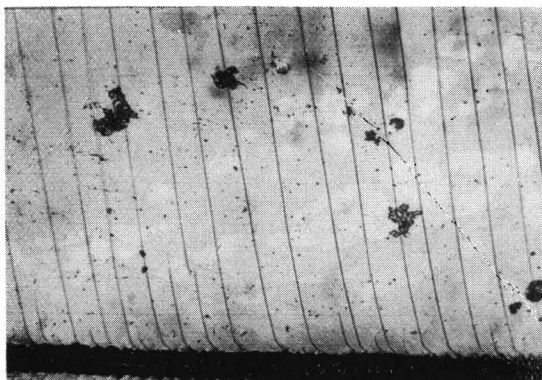
Photo. 21. Optical micrograph of test specimen No. 23. Black band underneath is the marked line perpendicular to the slip bands. 77 \times
