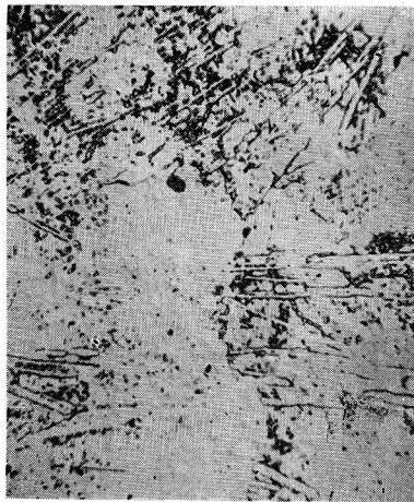
Photo. 14 \times 300 C=0.50%, As=10.05% Annealed structure, 5% Picral etch. Ferrite+Pearlite. (Pearlite-cementite is partly spheroidized.)
