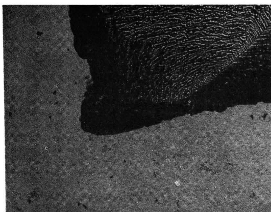
Photo 19 Electron micrograph of the alloy containing 1.52% Mg, 8.47% Zn and 1.57% Cu, aged at 100°C. for 5 hrs. Etched with Lacombe's reagent. Showing the distinct precipitation on the edges of steps in the surface of a large etch pit and the indistinct precipitation at the grain boundary. \times 10,000
