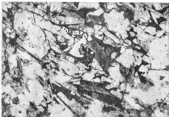
Photo 43. 2-1 Sample after melted. \times 180 (polished surface)
