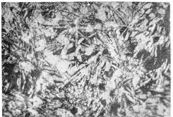
Photo 42. 3-1 Sample after melted. \times 180 (polished surface)
