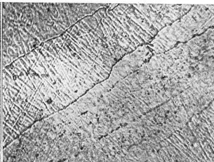
Photo 2. Ti 45.06% Fe, 54.16% alloy. Water-quenched after annealing 120 hrs at 1000^\circ C . Single phase of TiFe . Etchant: 20% HF, 20% HNO_3 in glycerine.
