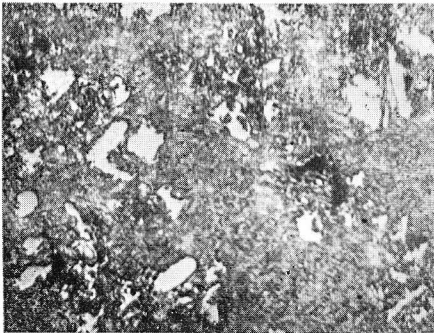
Photo 28. Ti 24.25%, Fe 71.61%, C 6.00% alloy. As Cast. Primary \delta plus Eutectic (TiC + \alpha -Fe). Etchant: Picral.
