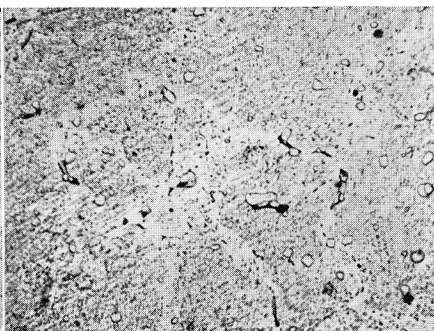
Photo 6. Ti 47.03%, Fe 51.81% alloy. Water-quenched after annealing 900 hrs at 800^\circ C . Single phase of TiFe . Etchant: 20% HF, 20% HNO_3 in glycerine.
