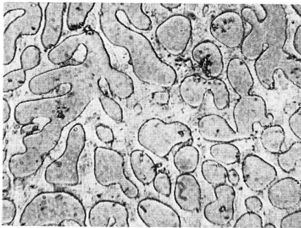
Photo 21. Ti 58.45%, Fe 37.02%, C 5.71% Alloy. As Cast. Primary \delta plus TiFe. Etchant: 20% HF, 20% HNO 3 in glycerine.
