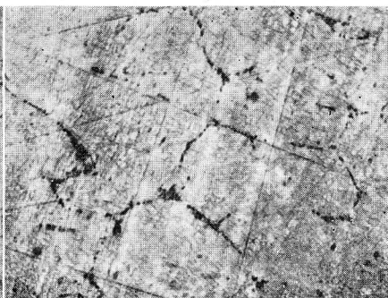
Photo 10. Ti 32.36% Fe 68.54% alloy. Water-quenched after annealing 70hrs at 1000°C. Single phase of TiFe 2 . Etchant: 20% HF, 20% HNO 3 in glycerine.
