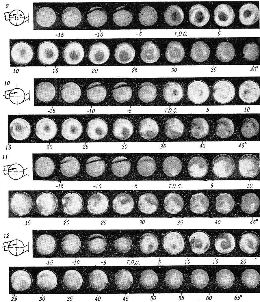
Fig. 9 Examples of high-speed photographs taken at various connecting passage area ratios, and taken at varying engine speeds
