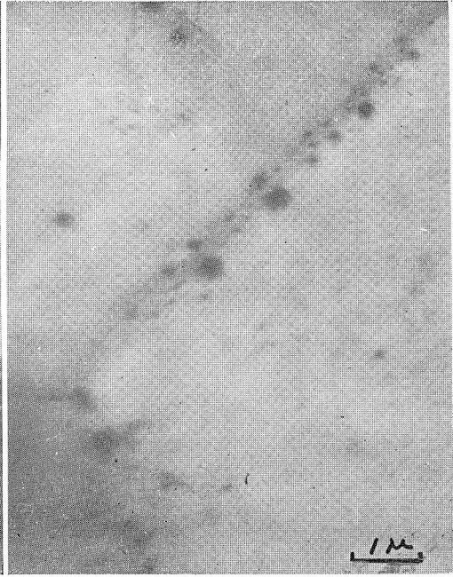
Photo. 25. Mg-1.7%Th alloy, W.Q., aged for 3 hr at 250°C, showing preferential precipitates on the grain boundaries. ( \times 10,000 )
