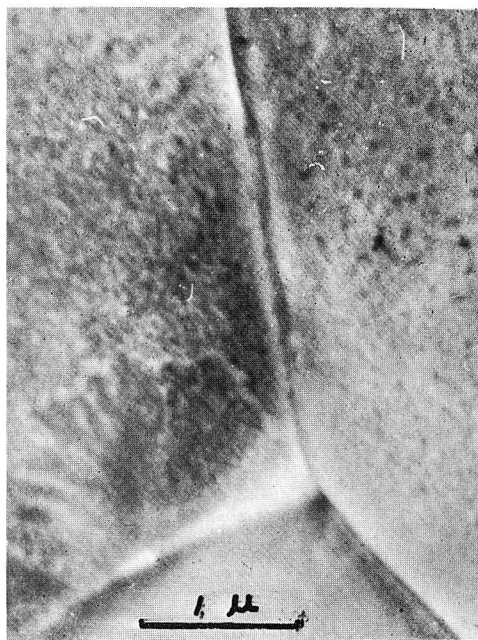
Photo. 11. Al-28.3% Zn alloy, W.Q., aged for 1 hr at 150°C. \times 21,000 .
