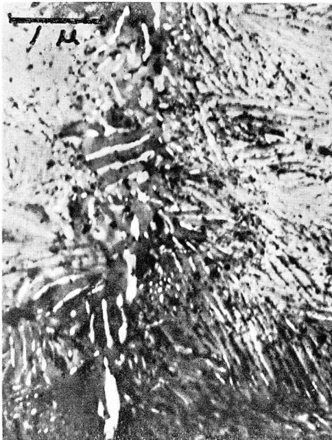
Photo. 17. Al-40.8% Zn alloy, W.Q., aged for 3 hr at 150°C. \times 17,500
