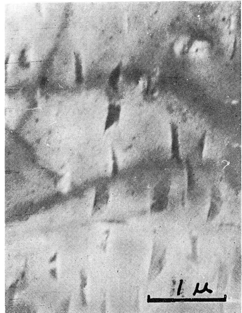
Photo. 19. Al-28.3% Zn alloy, quenched from 300°C, aged for 1 hr at 250°C. Showing precipitates having a large size thought to be equilibrium zinc phase. \times 21,000
