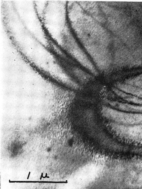
Photo. 33 Al-Cu-Zr alloy, W.Q., aged for 1 day at 150°C. ×25000
