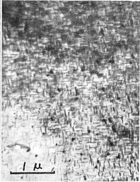
Photo. 52 Al-Ag-Zr alloy, W.Q., 20% rolled, aged for 4 hrs at 200°C. \times 20000
