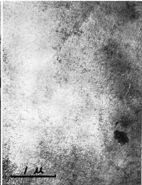
Photo. 46 Al-Ag-Zr alloy, W.Q., aged for 4 days at 110°C. \times 20000
