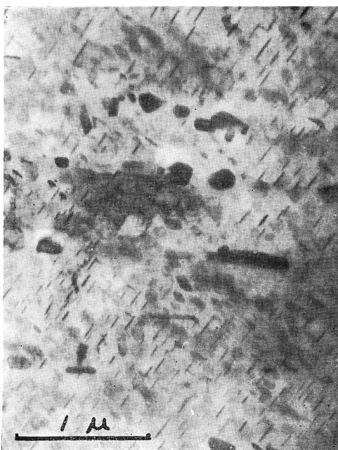
Photo. 29 Al-4% Cu alloy, W.Q., 40% rolled, aged for 1 day at 200°C. \times 25000
