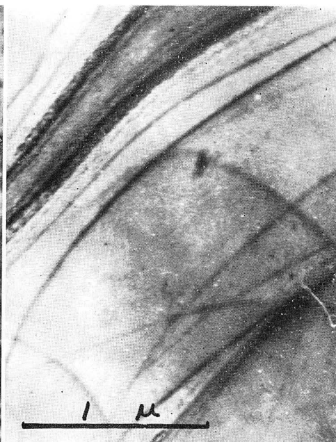
Photo. 24 Al-4% Cu alloy, W.Q., 5.0% elong., aged for 4 days at 110°C. \times 35000
