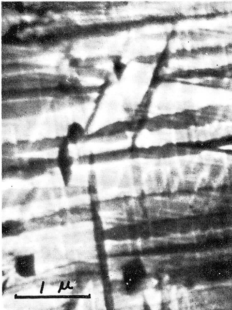
Photo. 49 Al-20% Ag alloy, W.Q., aged for 4 hrs at 200°C. ×20000
