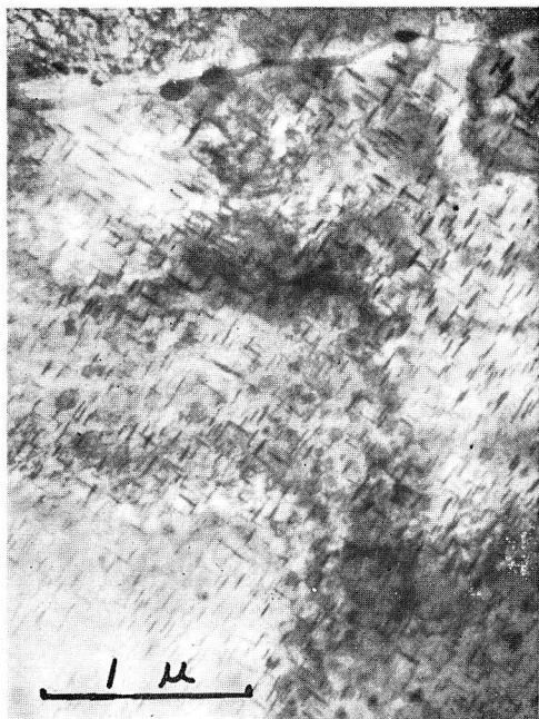
Photo. 35 Al-Cu-0.3% Be alloy, W.Q., 5.0% elong., aged for 1 day at 200°C. \times 25000
