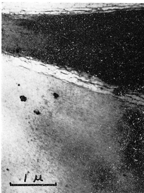
Photo. 41 Al-20% Ag alloy, W.Q., aged for 1 day at 110°C. \times 20000
