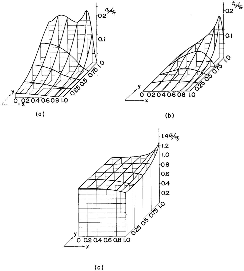
Fig. 5. Stresses in the specimen with height/width=1.0
