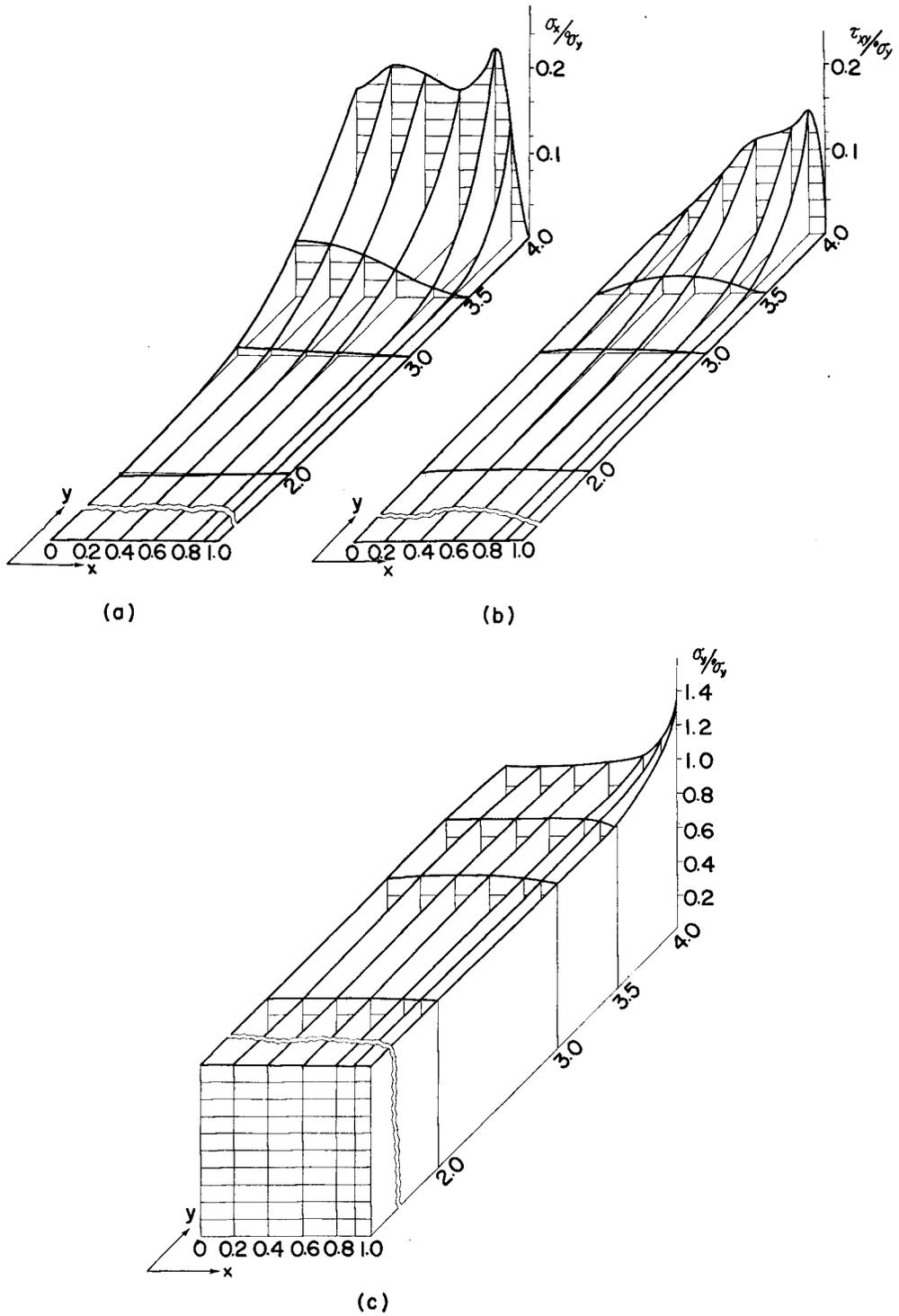
Fig. 7. Stresses in the specimen with height/width=4.0.
