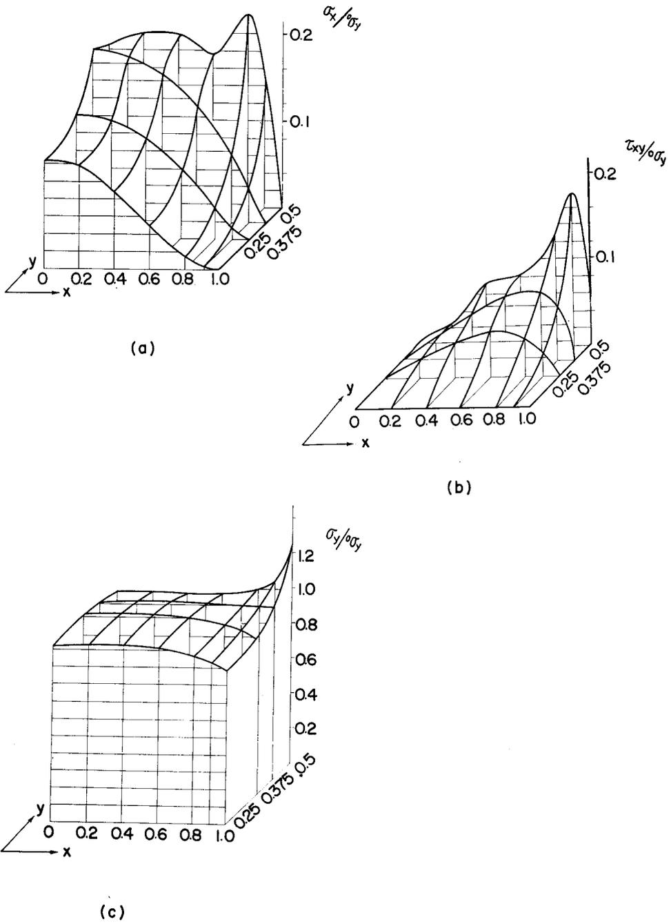
Fig. 4. Stresses in the specimen with height/width=0.5.
