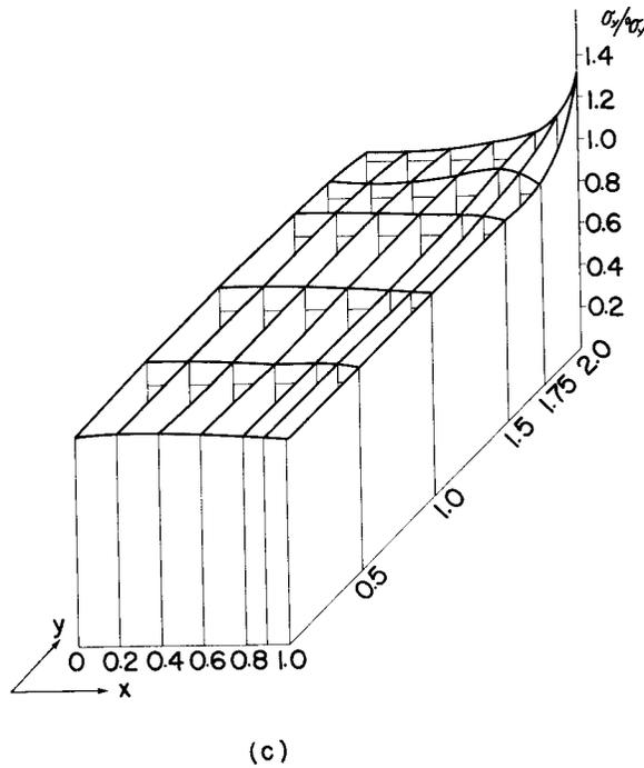
Fig. 6. Stresses in the specimen with height/width=2.0.
