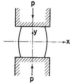
Fig. 2. Rectangular block after compression.
