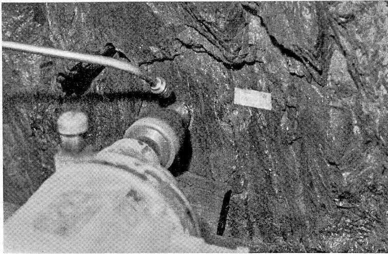
Fig. 5. Overcoring in the field using an electric hand drill.
