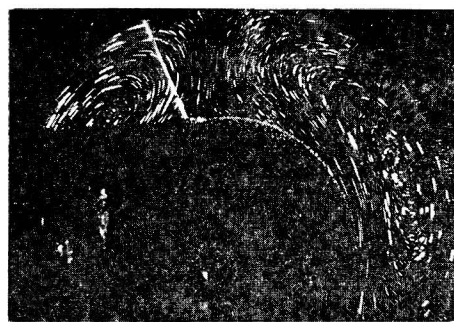
Fig. 9. Flow pattern of convection current ( \theta_1 - \theta_2 = 3^\circ\text{C} )
